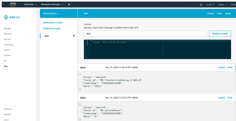
Congratulations! You have successfully sent your Modbus or CAN bus data to your AWS IoT endpoint and ready to, for example, push the data to a S3 bucket using a Rule in 'Act > Rules'. The FATBOX G3 AWS IoT client side is built using AWS IoT Device SDK for Python and users are free to install, modify our device client codes for enhanced edge capabilities or other required functionalities.
